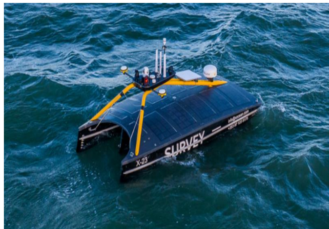
Figure 2: USV with hull mounted sensors
